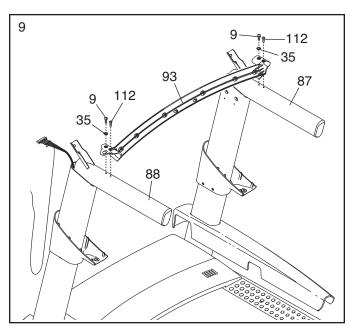
10. With the help of a second person, hold the console assembly near the Left Handrail (88).
